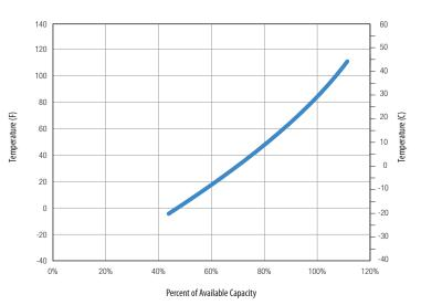
E. C.A. (Cranking Amps) - the discharge load in amperes which a new, fully charged battery can maintain for 30 seconds at 32°F (0°C) at a voltage above
